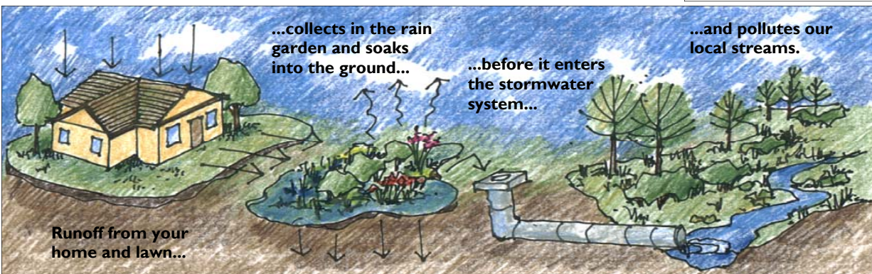
In this diagram, arrows show the path of runoff from home and lawn to rain garden, stormwater system, and stream. Rain gardens catch pollutants before they reach our streams.
