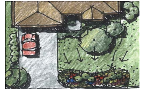
A plan of a typical front yard rain garden. The garden is located to catch runoff from the lawn and rain gutters.
